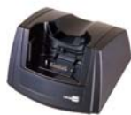
Charging and communication cradle/ Ethernet cradle
