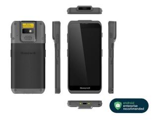
Android 11, 5.5-inch Corning Gorilla Glass touchscreen, Qualcomm Snapdragon octa-core 2.0GHz processor, Wi-Fi 5, Bluetooth 5.1, 4G LTE connectivity, one nano SIM plus one eSIM, IP67.
