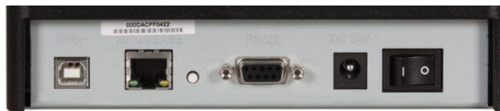
On-board LAN, USB and Serial interfaces
