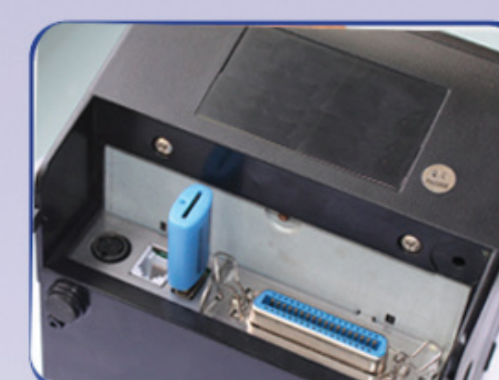
Firmware updating by USB memory stick
