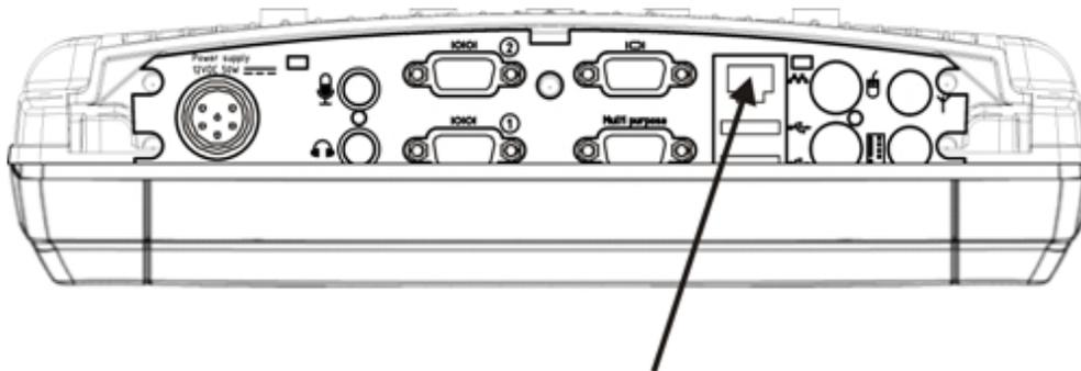
1. Insert the network cable and ensure it is firmly seated in the connector jack.
