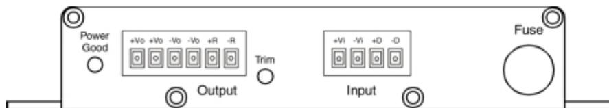
Attach the stripped wire ends to the output side of the DC to DC converter. Attach stripped wire ends to the input side of the DC to DC converter.
