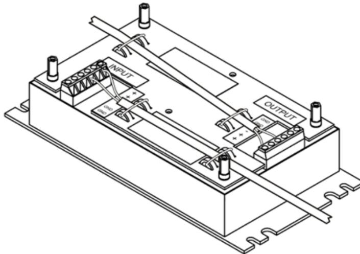
Remove the lid from the DC to DC converter. Attach the stripped wire ends to the output side of the DC to DC converter. Attach stripped wire ends to the input side of the DC to DC converter.
