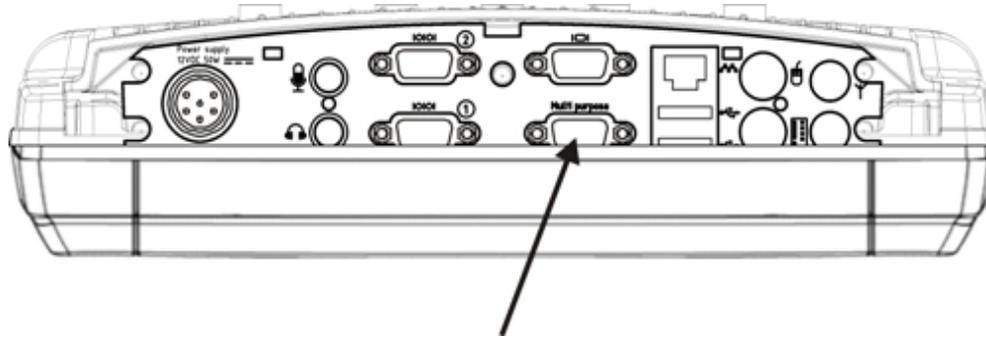
1. Seat the cable connector firmly over the pins and turn the thumbscrews in a clockwise direction. Do not overtighten.
