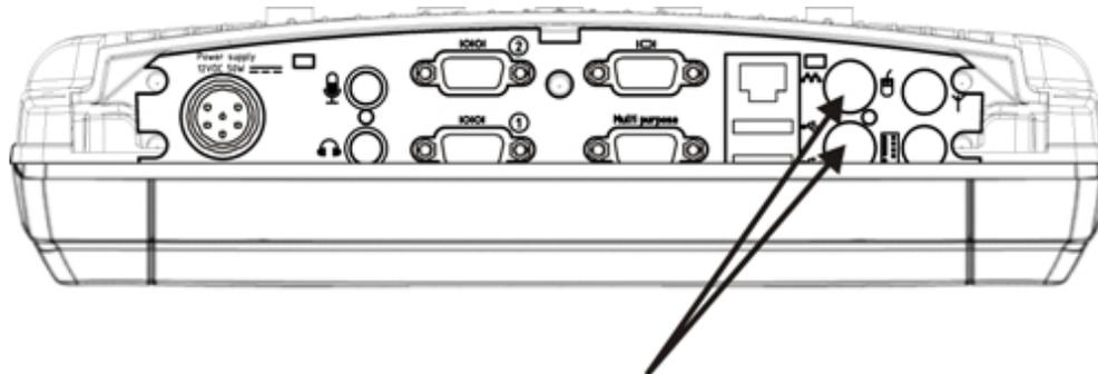
1. Connect the adapter cable to the PS/2 connectors on the Thor VX8.
