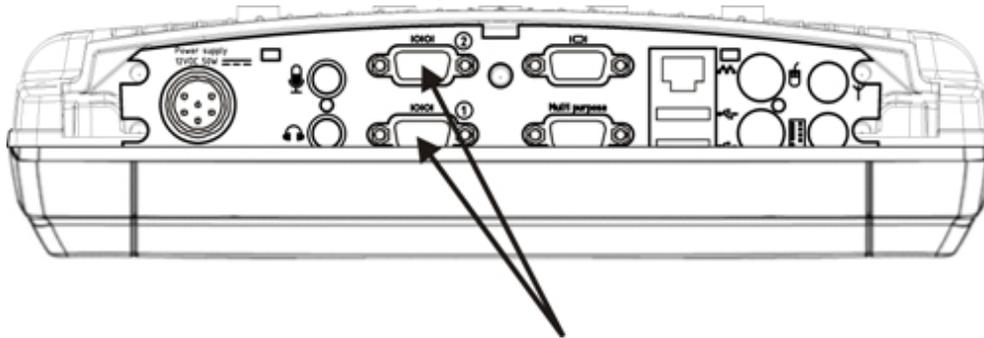
Seat the connector firmly over the pins and turn the thumbscrews in a clockwise direction. Do not overtighten.
