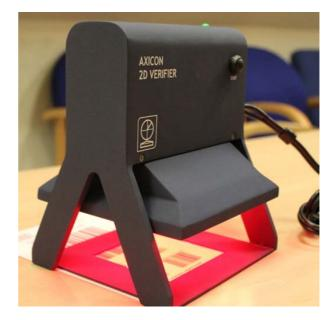
The Axicon 12600 verifier for 2D and linear barcodes with a maximum size of 51mm x 38mm
