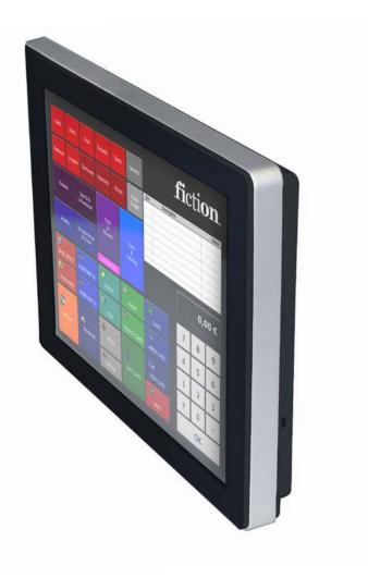
This 'all-in-one' touchscreen system is fanless and features a slimline design as well as a splash-proof front. Easy to install anywhere and ideal for wall-mounted till operations, it can also be mounted on a pole (or placed on a stand).
